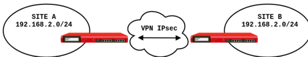
Figure 1.1: VPN IPsec between two geographically distant locations.
